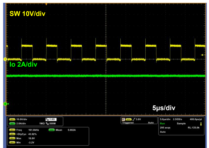
Figure 11-11. Switching Waveform ( V_{in}=12V , V_o=5V , I_o=5A )
