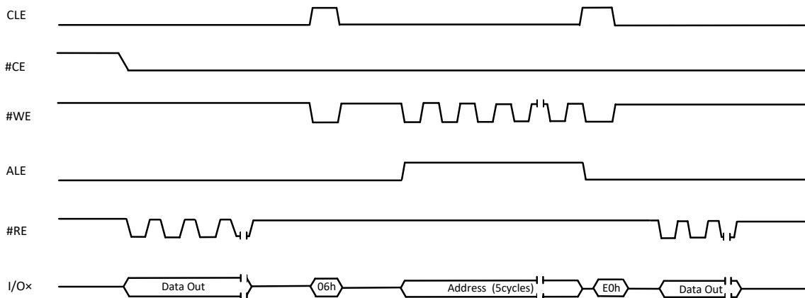
Figure 9-4 Two Plane Random Data Read (06h-E0h) Operation
