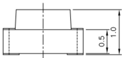
For reflow soldering (Propose)
