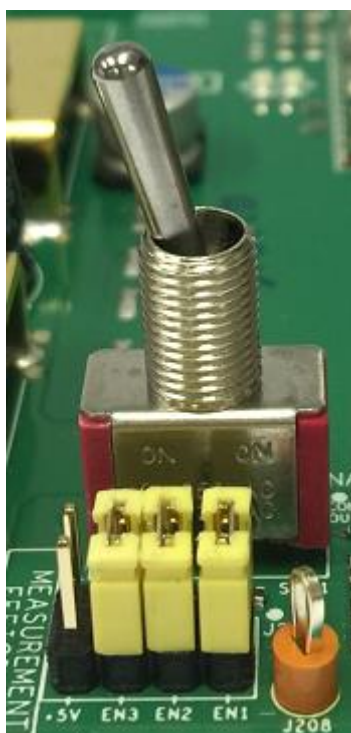
Fig. 4 – Enable jumper location and population
