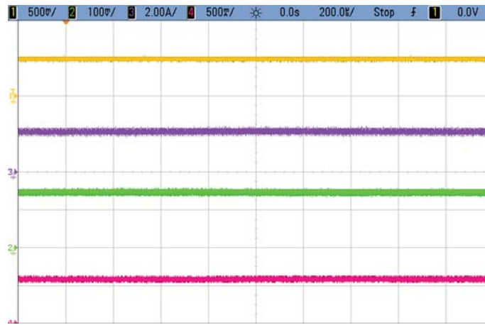
Figure 7. Input and Output Current Monitoring V_{IN} = 12V , I_{IN} = 620mA , V_{OUT} = 3.3V , I_{OUT} = 2A , f_{SW} = 1MHz Trace 1: I_{OUTMON} Voltage (0.5V/DIV) Trace 2: I_{INMON} Voltage (0.1V/DIV) Trace 3: I_{OUT} Current (2A/DIV) Trace 4: I_{IN} Current (500mA/DIV)
