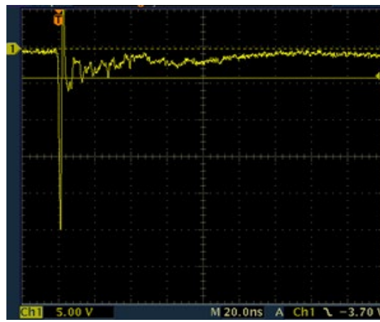
SP1105S IEC 61000 -4-2 -8 kV Contact ESD Clamping Voltage
