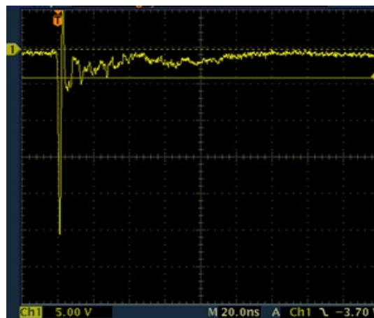
SP1112 IEC 61000 -4-2 -8 kV Contact ESD Clamping Voltage
