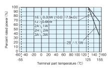
When the terminal part temperature of the resistor exceeds the rated terminal part temperature shown above, the power shall be derated according to the derating curve. Please refer to "Introduction of the derating curves based on the terminal part temperature" on the beginning of our catalog before use.
