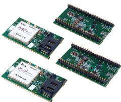
engine. The LTE910CF v7.00 units operate in LTE bands (B13), (B12), (B5), (B4) and (B2), with fallback to HSPA+ networks as needed. End device certification allows users to implement the LTE910CF in their devices with no further North American carrier certification requirements
