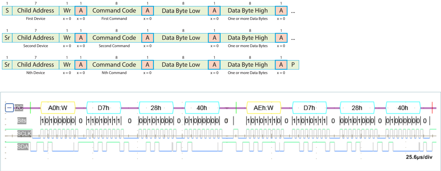
Figure 33 — DISABLE_FAULT COMMAND (D7h)_WRITE
