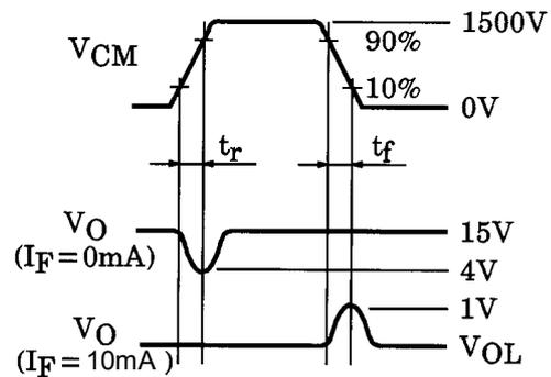
$$CM_H = \frac{1200(V)}{t_r(\mu s)}, \quad CM_L = \frac{1200(V)}{t_f(\mu s)}$$
