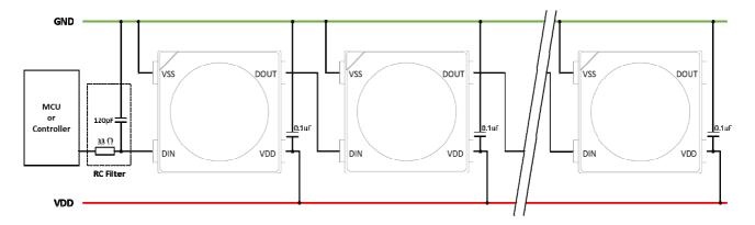
Cascading connection for normal driver IC embedded LEDs is shown. The data signal is transmitted one-by-one. The output of the previous one is connected to the input of the next one. As for the power positive and negative, all LED positives should be connected to VDD and all LED negatives should be connected to ground.
