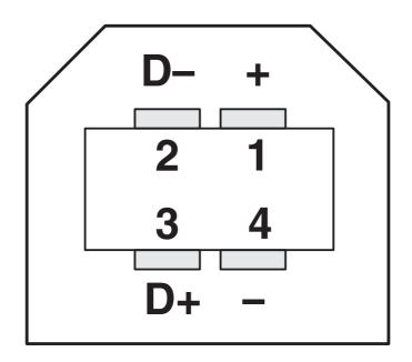
Plug pin assignment plug USB, type B
