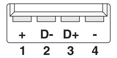
Pin assignment plug USB, type A
