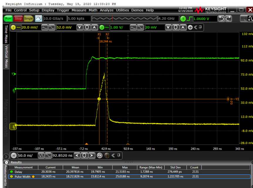
Figure 40. Typical Laser Optical Pulse Shape
