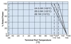
For resistors operated at a terminal part temperature of described for each size or above, the power rating shall be derated in accordance with the above derating curve. Please refer to "Introduction of the derating curve based on the terminal part temperature" in the beginning of our catalog prior use.
