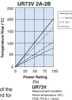
Regarding the temperature rise, the value of the temperature varies per conditions and board for use since the temperature is measured under our measuring conditions.
