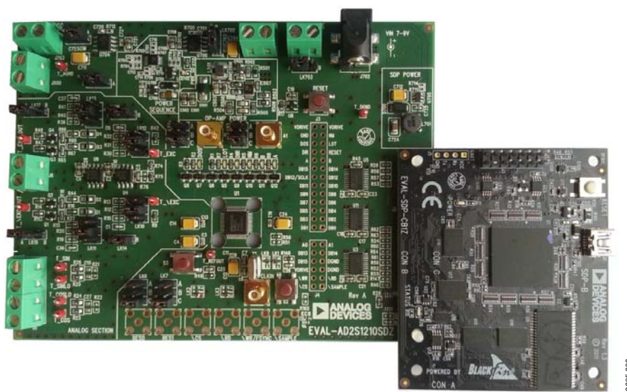
Figure 2. Evaluation Board (Left) Connected to the SDP Board (Right)
