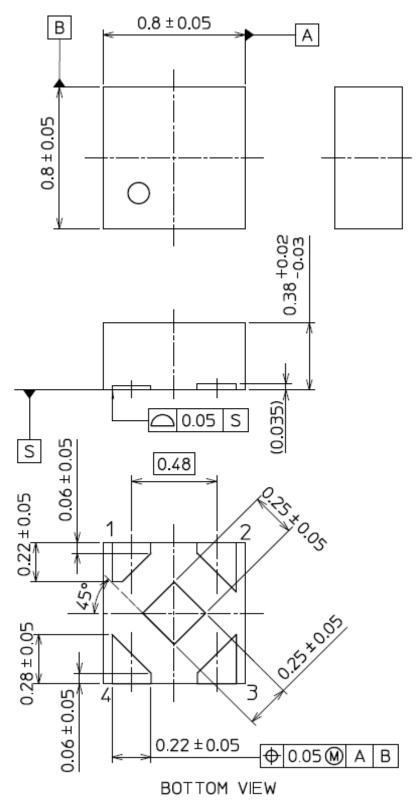
0.04 mm (typ.) unevenness exists along the edges of the back electrode to increase shear after soldering.
