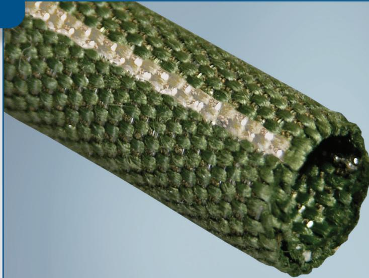
**ROUNDIT® 2000 MA** is a woven combination of meta-aramid and PPS (poly-phenylene sulfide). The meta-aramid/PPS blend in a flat weave construction gives ROUNDIT 2000 MA a rugged yet smooth texture and appearance for high temperature bundling and abrasion resistance. This product is rated to +200°C (+392°F) and is non-halogenated.
