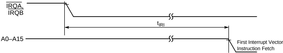
Figure 10-8 Interrupt from Wait State Timing
