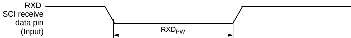
Figure 10-16 RXD Pulse Width
