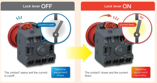
\* The example shows an NC contact. However, all contacts are interlocked with the lock lever, and the statuses of NO contacts are also switched
