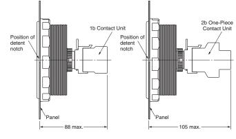
Push-in Plus Terminal Block Type Mounting a 1-pole Switch Unit \*
