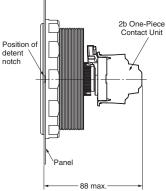
\* These are the dimension from the front of the panel when the Switch Unit is attached.
