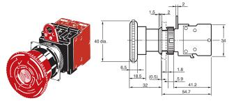
Note: Unless otherwise specified, a tolerance of ±0.8 mm applies to all dimensions.
