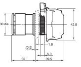
A22NE-L-P 2-N Large Turn-reset (60-dia.) Degree of Protection: IP65 oil-resistant models
