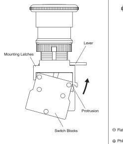
(2) Removing the Switch Blocks
