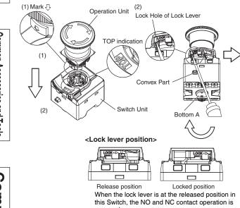
reversed. Set the lock lever to the locked position when using the Switch.
