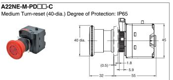
Note: Unless otherwise specified, a tolerance of ±0.8mm applies to all dimensions.
