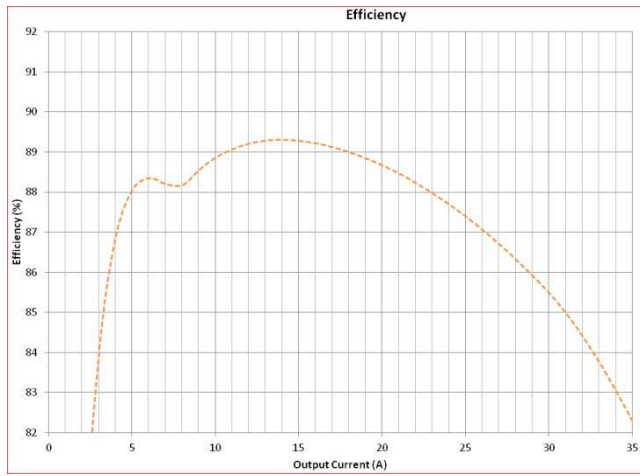
Figure 5. Efficiency – 19 V Input, 1.2 V Output, 500 kHz
