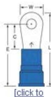
This terminal has a wire range of 6 AWG and a stud size of 10. It comes in quantities of 200 per case.
