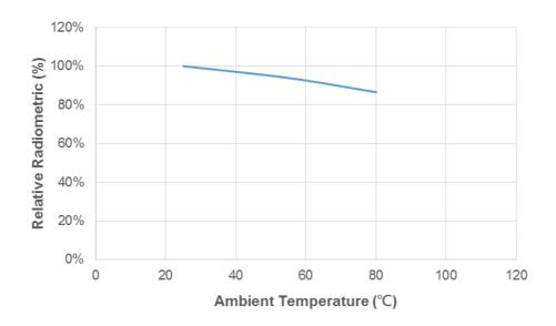
Fig.4 Relative Radiant Flux vs Ambient Temperature
