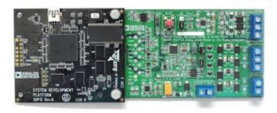
The **EVAL-CN0202-SDPZ** board provides a full function, high voltage (up to 44 V), flexible, programmable analog output solution that meets most requirements for programmable logic controller (PLC) and distributed control system (DCS) applications. When using this evaluation board with the SDP board or BeMicro SDK board, apply +6 V and GND to Connector CN2, 12-50 V and GND to Connector CN3.
