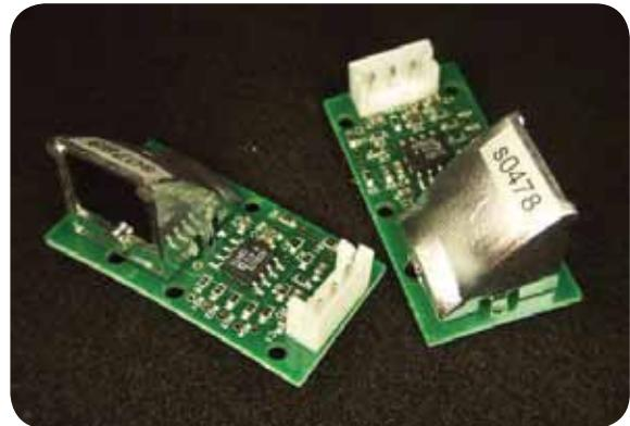
The ZTP-115M is a single IR module used for non-contact surface temperature measuring. It consists of a thermopile, IR sensor, signal conditioning and voltage output.
