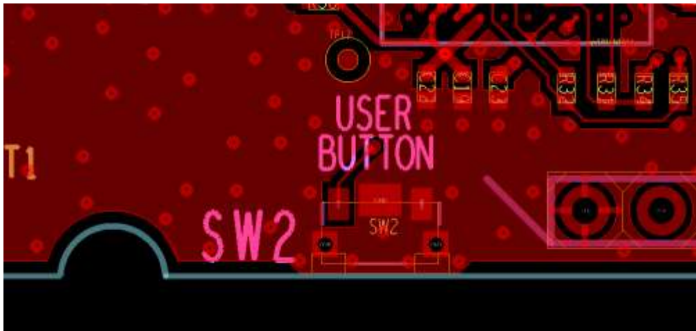
Figure 15: General Purpose Push Button SW2
