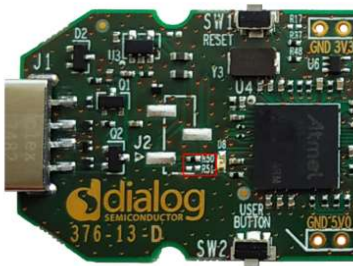
Figure 28: Resistors R50 and R51
