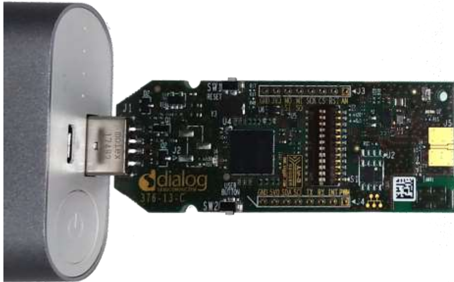
Figure 26: Operation with a Battery Pack
