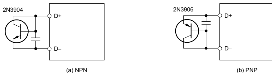
Figure 7-6. Remote Temperature Sensor Using Transistor
