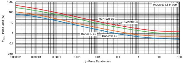
Maximum pulse load, single pulse; applicable if  $\overline{P} \rightarrow 0$  and n < 1000 and  $\hat{U} \le \hat{U}_{max}$ ; for permissible resistance change equivalent to 8000 h operation
