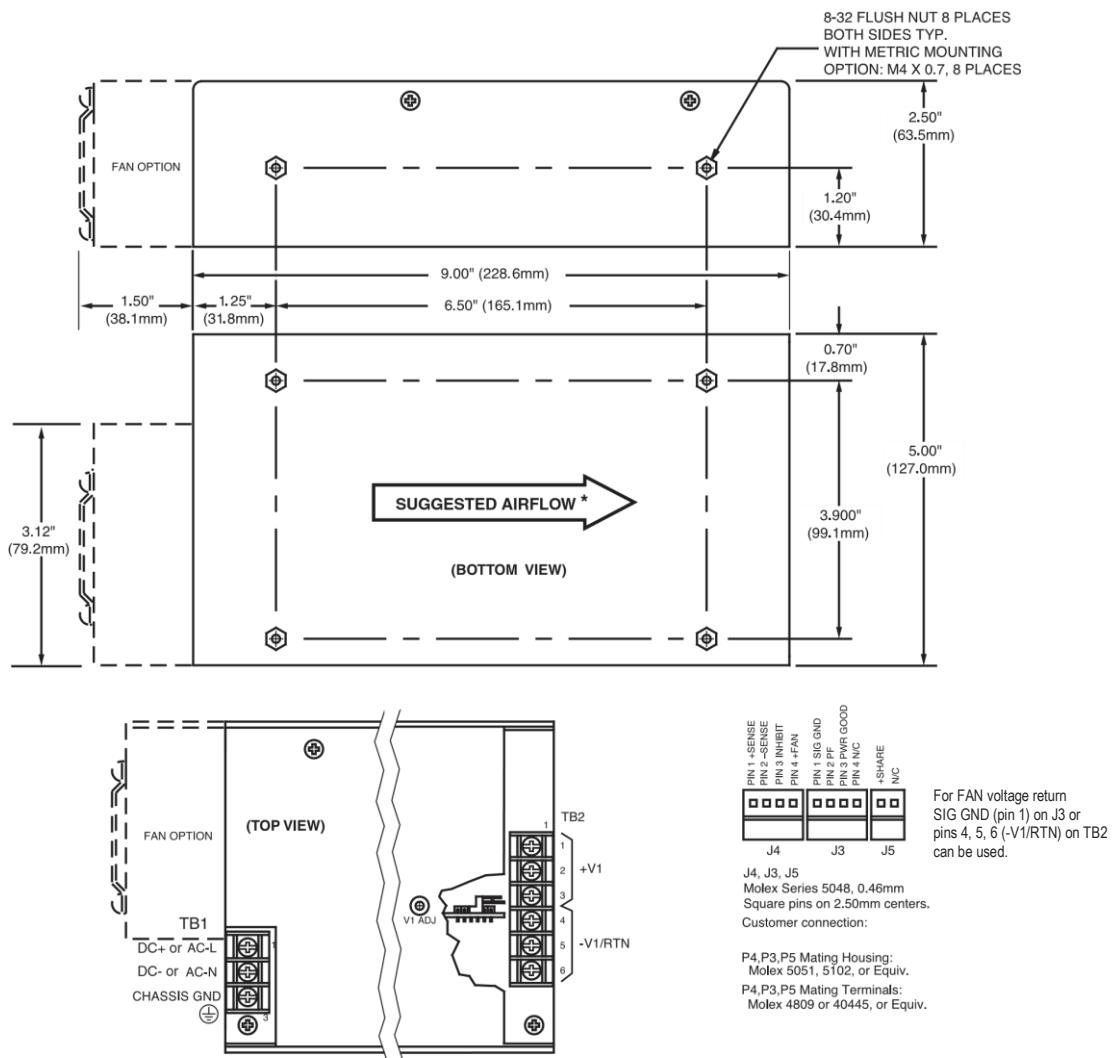
Figure 1. Mechanical Drawing of PFC500 model
