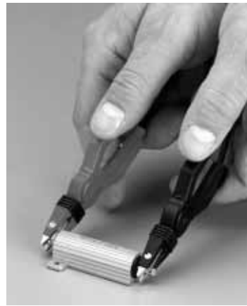
Four-wire measurement with only two clamps.
