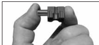
Touch-protected in the unplugged condition, not valid for the longer plug.
