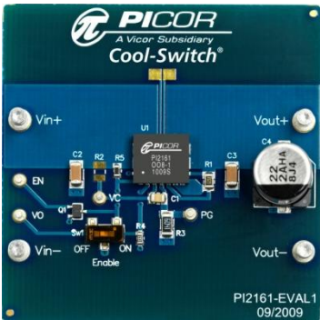
Figure 1: PI2161-EVAL1 Evaluation Board (1.8" x 1.8")
