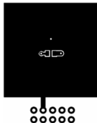
a) 80^\circ\text{C/W} when mounted on a 1\ \text{in}^2 pad of 2 oz copper
