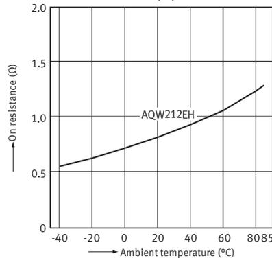
2-3. On resistance vs. ambient temperature characteristics
