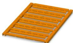
Marker for terminal blocks, Sheet, orange, unmarked, can be labeled with: BLUEMARK E.CARD, BLUEMARK ID COLOR, BLUEMARK ID, BLUEMARK CLED, THERMOMARK PRIME 2.0, THERMOMARK PRIME, THERMOMARK CARD 2.0, THERMOMARK CARD, TOPMARK NEO, TOPMARK LASER, mounting type: latching, for terminal block width: 10.2 mm, Number of individual labels: 36, text field height: 4.7 mm, text field width: 9.4 mm
