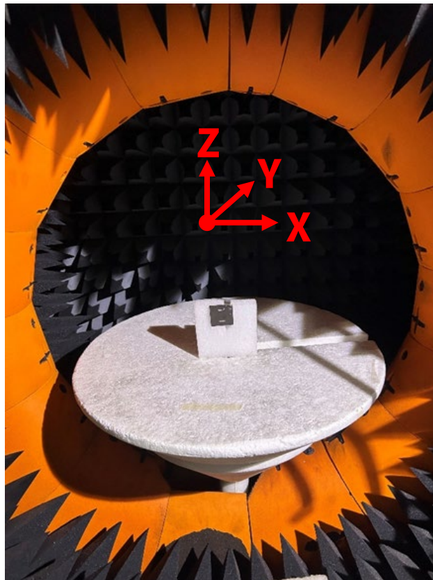
Chamber Test Setup
