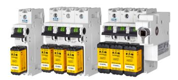
The DIN-Rail mounted 1-, 2- and 3-pole Compact Circuit Protector (CCP2\_CF) is a UL 98 horsepower rated disconnect available in 30, 60 and 100 A ratings. Each CCP will accept a fuse amp rating equal to or less than its rating. These switches are also available in rotary versions for through-the-door or through-the-side operation. Accessories include multi-wire lug kits with terminal shrouds, auxiliary contacts and PLC fuse monitor (see data sheet no. 1157).
