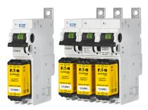
The 1-, 2- and 3-pole Compact Circuit Protector Base (CCPB) is a UL 98 horsepower rated branch circuit disconnect. Primarily used in the Quik-Spec Coordination Panelboard, it's available in ratings up to 100 amps. The CCPB has amp rejection breaks at 15, 20, 30, 40, 50, 60, 70, 90 and 100 amps that coincide with standard conductor ampacities to help prevent overfusing by rejecting any CUBEFuse amp rating greater than that of the switch
