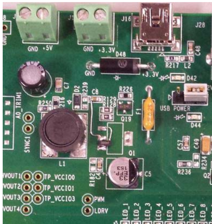
Figure 43. Q1 Package Change and Connections
