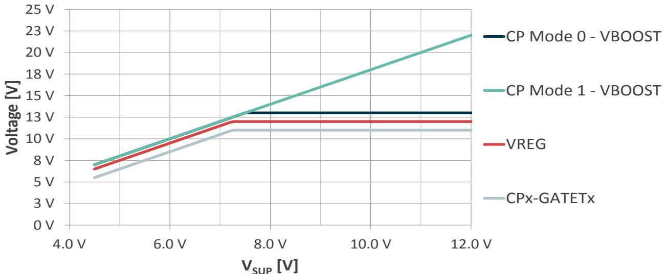
Figure 12-3 Charge pump output and driver supply
