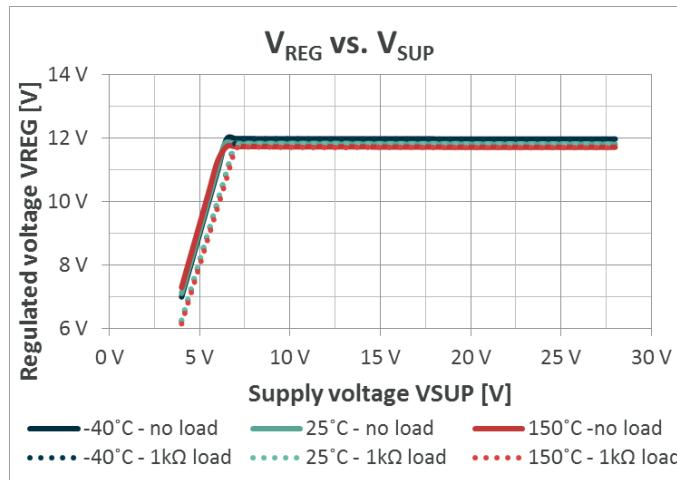
Figure 10-1 MLX83100 Regulated output voltage vs. supply voltage
