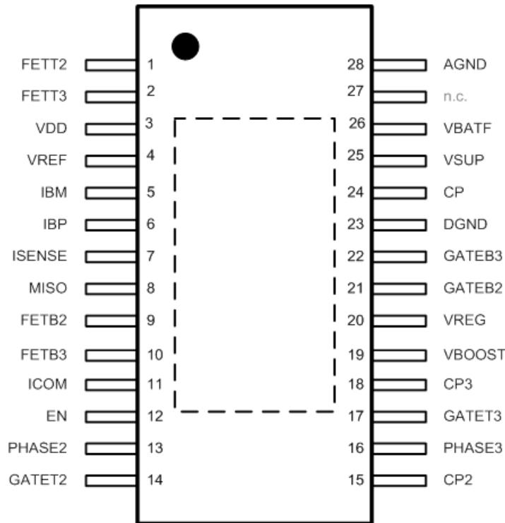
Figure 7-1 Pin configuration
