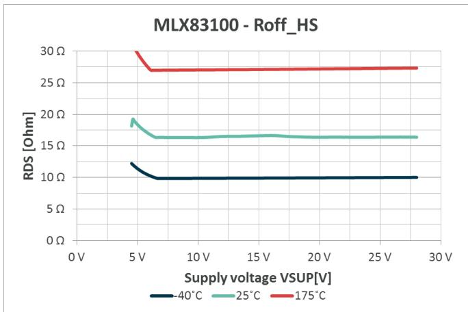
Figure 10-4 MLX83100 High-side driver FET R<sub>OFF</sub> resistance vs. supply voltage
