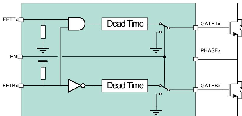
Figure 12-5 Input control logic of the driver stage
