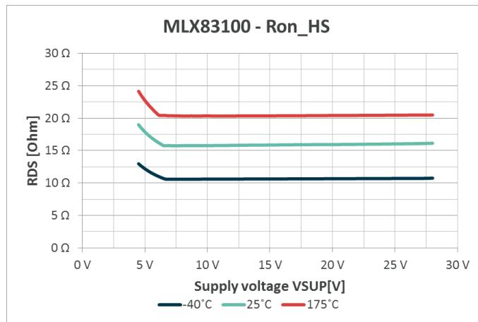
Figure 10-3 MLX83100 High-side driver FET R<sub>ON</sub> resistance vs. supply voltage
