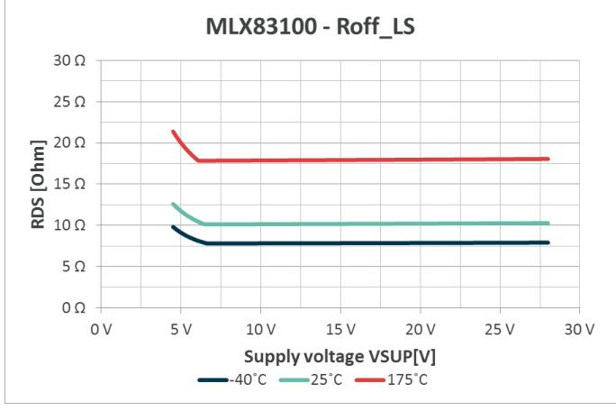
Figure 10-6 MLX83100 Low-side driver FET R<sub>OFF</sub> resistance vs. supply voltage
