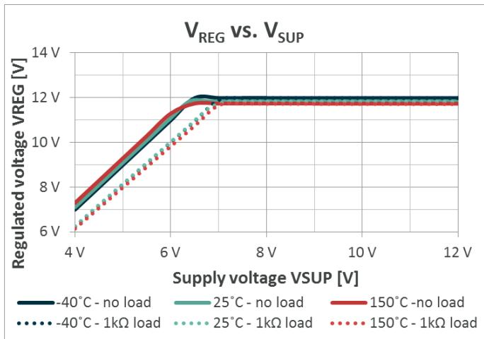
Figure 10-2 MLX83100 Regulated output voltage vs. supply voltage
