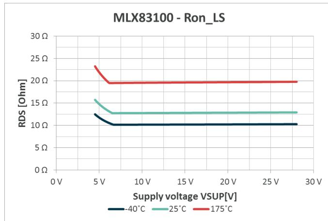
Figure 10-5 MLX83100 Low-side driver FET R<sub>ON</sub> resistance vs. supply voltage
