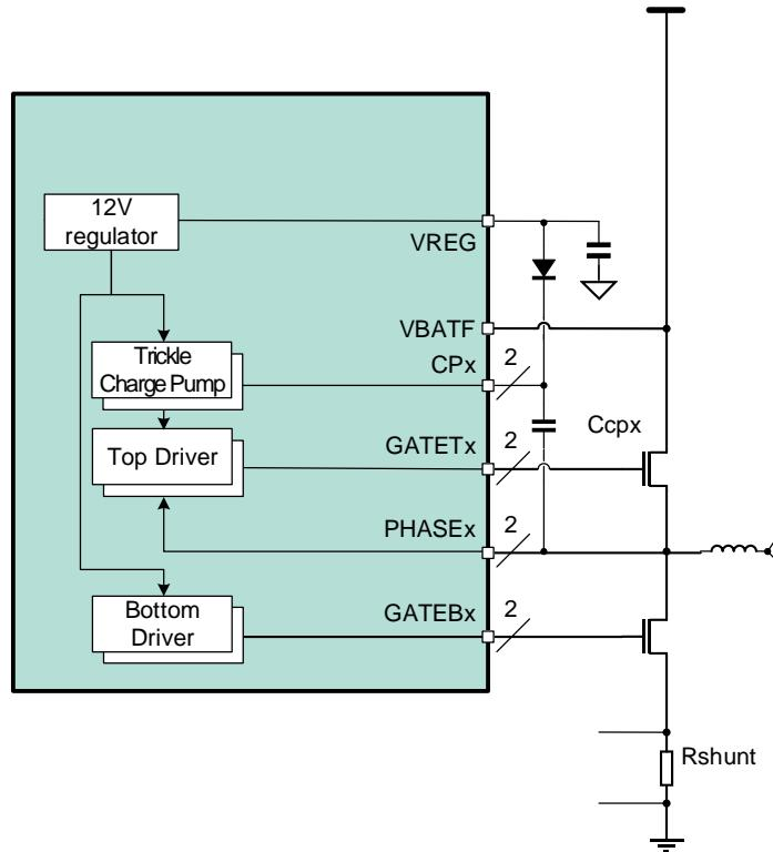
Figure 12-4 Voltage regulator for driver supply – VREG
