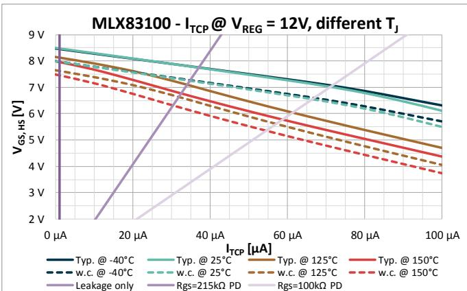
Figure 10-8 MLX83100 Trickle charge pump current capability vs gate drive voltage at different VREG, at 150°C
