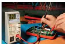
Current limited DC supply for electronic repair and calibration
