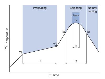
Preheating Soldering Peak Temp. Time Temp. Time Temp. Time T1 T2 t1 тз t2 Т4 t3 150°C 180°C 90 to 120s 230°C 40s 255°C 10s max.
