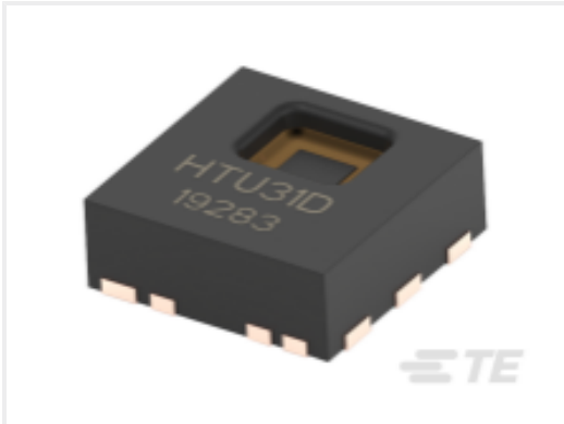
TE Part #10142048-20 HTU31D I.C 31D RH/T DIGITAL R400
