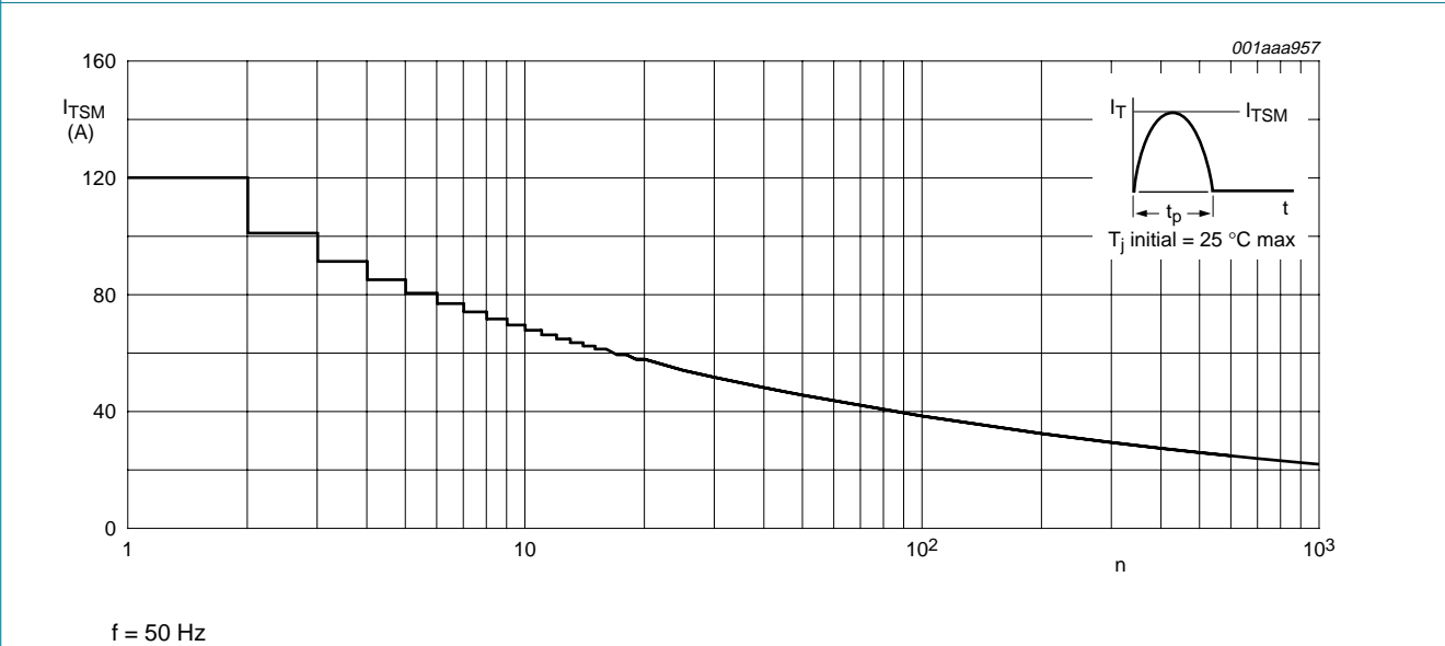
Fig 2. Non-repetitive peak on-state current as a function of the number of sinusoidal current cycles; maximum values
