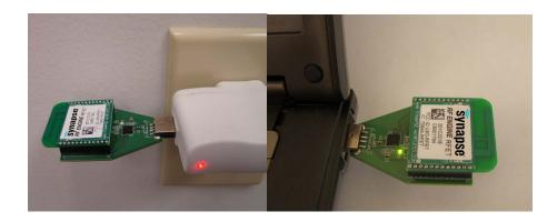
Note: The Portal software doesn't need to be installed for the SNAPstick to draw USB power.
