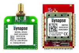
Each SNAP Engine combines a microcontroller, a radio, and an antenna. The antenna can either be an integral "F" antenna, or a mounting point for an external antenna. The SNAP Engines included in your EK2100 evaluation kit are RF100 SNAP Engines (also known as RF Engines), as pictured above. RF100 SNAP Engines communicate using 802.15.4 2.4 GHz radio signals.
