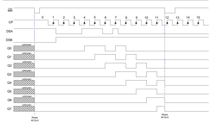
5. All Q values are reset to LOW when  $\overline{MR}$  goes low.  $\overline{MR}$  is asynchronous and overrides all other signals. 6. Serial data supplied at DSA and DSB is ANDED and transferred to Q0 on positive edge of CP. Notes:
