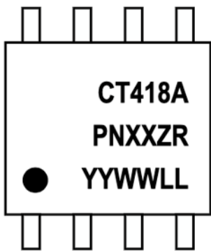
Figure 47: CT418 Device Marking for 8-lead Package
