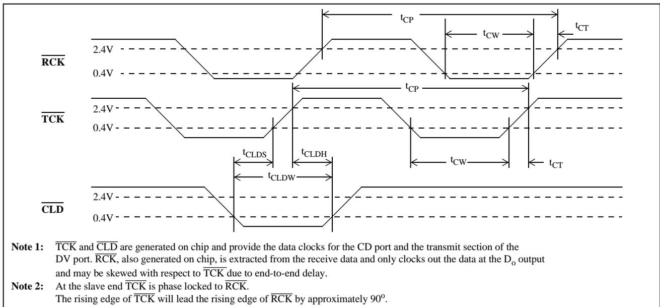
Figure 18 -  $\overline{\text{RCK}}$ ,  $\overline{\text{TCK}}$  &  $\overline{\text{CLD}}$  Timing For MOD Mode
