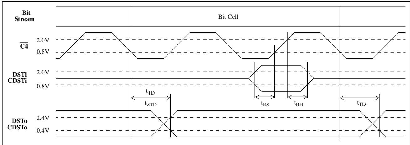
**Figure 19 - Data Timing For DN Mode**
