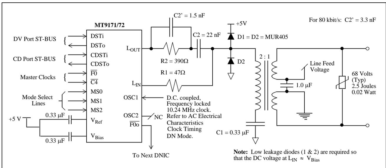
Figure 13 - Typical Connection Diagram - MAS/DN Mode, 160 kbit/s
