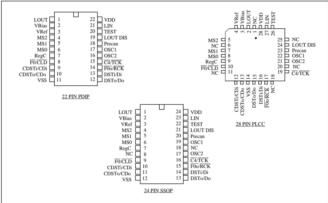
Figure 2 - Pin Connections
