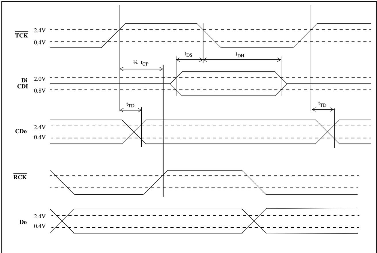
Figure 21 - Data Timing for Slave Modem Mode
