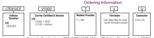
Example: Part Number – LTE910CFV1000TxUVN = LTE Cellular Plug-In Terminal; AT&T Certified; Telit Modem; Current Firmware with a U.F.L Connector with a Variable Voltage with no configuration options.
