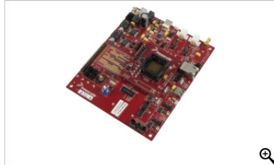
MPC574XG-MB Motherboard and MPC574XG-324DS Daughter Card
