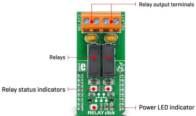
These relays are designed so that their coils can be easily activated by relatively low currents and voltages. For the G6D-1A-ASI DC5 relay operated at 5V, the coil current is 40mA. This makes them a perfect choice for activating them by an MCU. However, some additional components have to be included for a proper operation:
