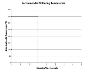
Soldering iron tip temperature should be set at 350°C (+10°C maximum), with the soldering duration not to exceed more than 3 seconds.
