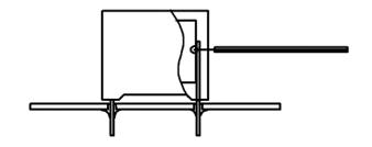
Temperature monitored inside the capacitor.
