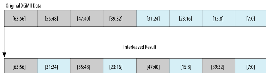
Figure 7-5: Interleaved SDR XGMII Data Mapping
